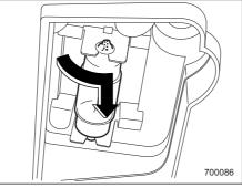
2. Turn the bulb until the flat surfaces at its ends are aligned vertically. Pull the
