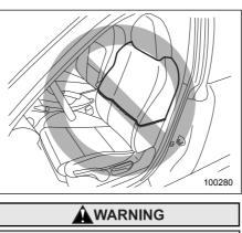
Do not put any kind of cover or clothes or other objects over either front seatback and do not attach labels or stickers to the front seat surface on or near the SRS side airbag. They could prevent proper deployment of the SRS side airbag, reducing protection available to the front seat's occupant.
